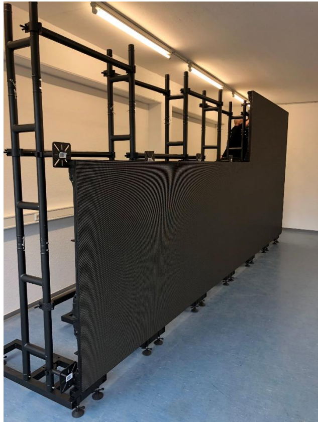
Ground Stack Installation
